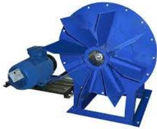
Figure 3. Centrifugal fan blade with a straight blade and a disc
